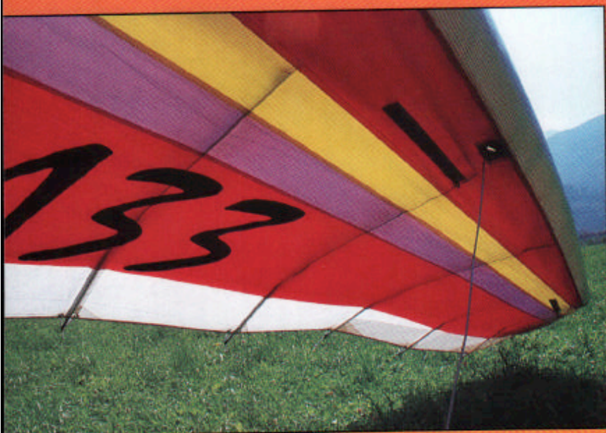
TOP: The Merlin lower surface showing no sag at the shear webs.
